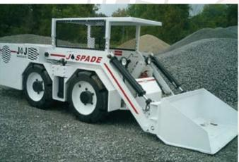
SETCO solid tires are the most advantageous in the mining industry. SETCO tires do not suffer from premature failures, which have plagued the mining industry. They are under no pressure whatsoever, eliminating the danger of the tire exploding or blowing out at the slightest puncture.
