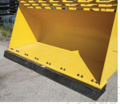
SETCO's rubber cutting edge protects and cleans the surface of the floor while effectively decreases tire spinning.
