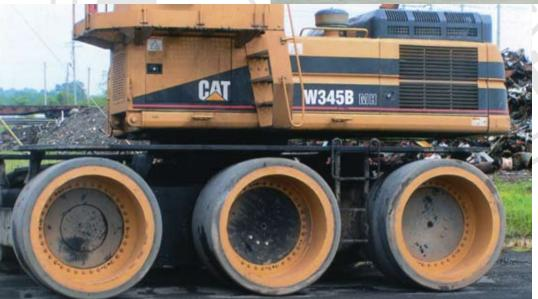
SETCO solid tires on a material handler will provide the durability and puncture resistance required to survive in a scrap yard environment.
