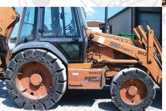
Solid tires for backhoes are the ideal solution by providing traction and increased pushing power. Rims are manufactured with A36 steel, combined with an exclusive rubber compound and compression molded, which provides extremely long life. The Soft Ride assembly offers a cushioned ride, with more comfort for the operator and less stress on the equipment.
