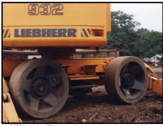
Due to the abusive environment that tires are exposed to in scrap yards, operators have found that SETCO Solid Tires are really the only option.
