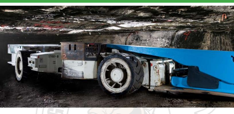
SETCO has the flexibility to custom manufacture solid tires to haul the heaviest loads and can easily change the entire dimensions of tires by varying the rubber depth for maximum load and carry. SETCO's custom heat dissipating rubber compound minimizes heat throughout the entire assembly to maximize load capacities.
