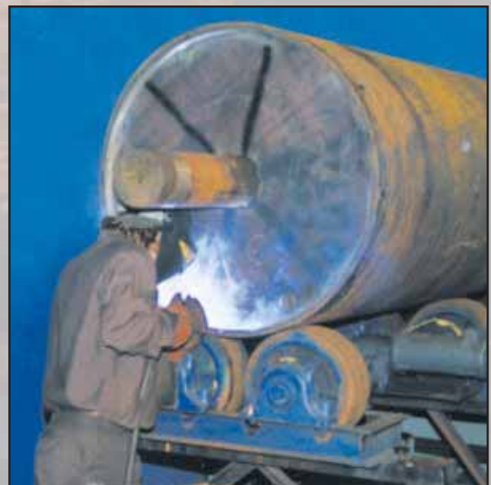
ROTATIONAL WELDING OF ROLL HEAD PLATE
