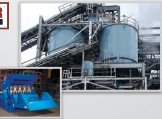
pneumatic conveyors, rotary airlocks, screens, chain and screw reclaimers, as well as metering and storage bins and silos.
